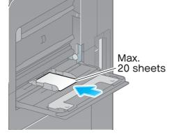
**NOTICE** When loading envelopes or postcards into the **Bypass Tray**, note the following points. → When loading envelopes, remove air from them, and securely press along the flap fold line. Otherwise, it will result in an envelope wrinkle or paper jam.
