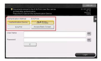
Check that [ID & Print/MFP Access] is selected in [ID & Print], and touch the Authentication Unit with your finger or IC card.
